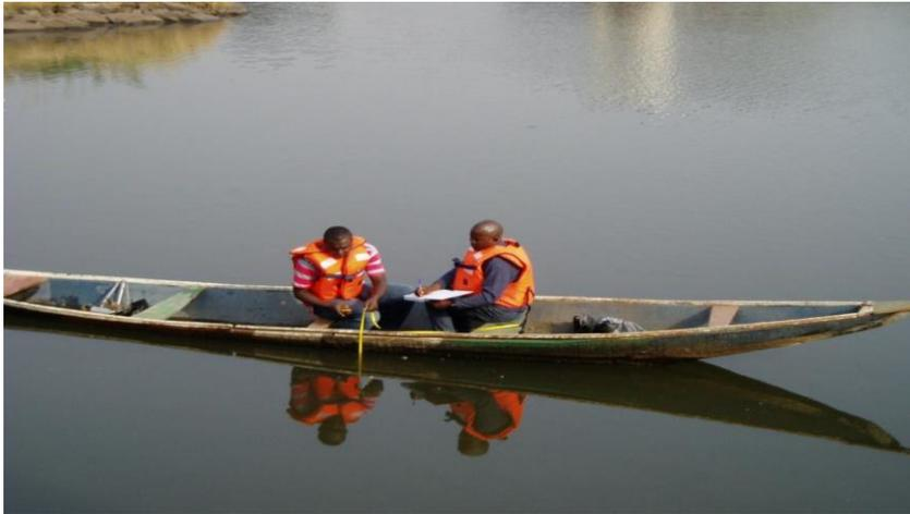
Figure 7: Depth measurement at the dam using lead-line
